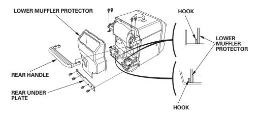
Install the lower muffler protector inside the hook securely.
