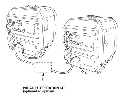
2. Start the generators (see page 22) and make sure the output indicator (green) on each generator comes on.
