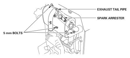
7. Use a brush to remove carbon deposits from the spark arrester screen.
