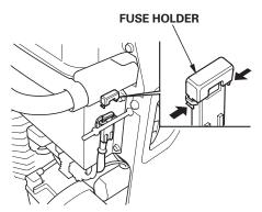
If frequent fuse failure occurs, determine the cause and correct the problem before attempting to operate the generator further.
