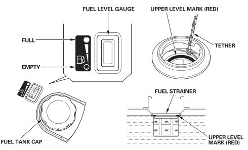
After refueling, reinstall the fuel tank cap securely.
