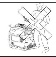
Always shut down the generator and allow it to cool before refueling!
