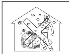
NEVER use a generator indoors! Exhaust and Carbon Monoxide can KILL YOU in minutes.
