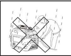
Avoid running the generator in the rain or very high, condensing humidity.
