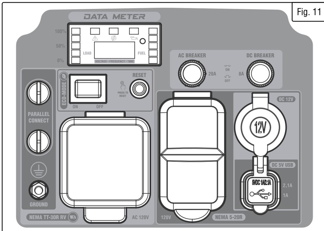
**NOTE:** The NEMA 5-20R receptacles are capable of connecting devices up to 20A only when two generators are parallel connected. When operating a single generator, do not exceed 15.8A (1900 running watts) on this receptacle.
