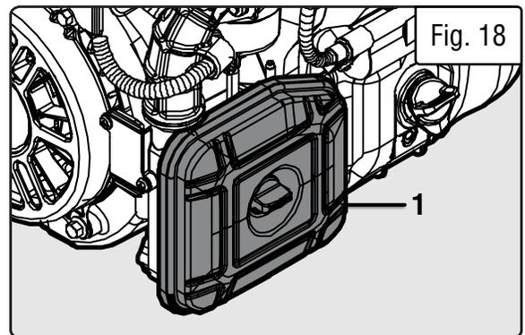
**⚠ CAUTION!** Running the engine with a dirty, damaged, or missing air filter element will result in possible danger and cause the engine to wear out prematurely.
