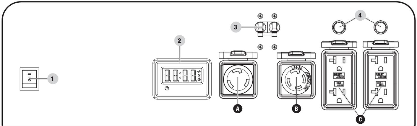
1. **Ignition Switch** – Used to START or STOP the generator.
