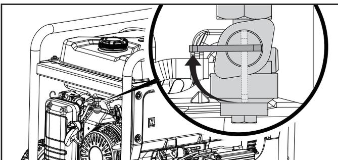
**Important:** Always ensure that the fuel valve and the ignition switch are in the "OFF" position when the generator is not in use.
