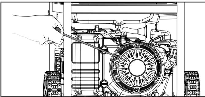
4. Do not over-choke. As soon as engine starts, move the choke to the "RUN" position over a 2-5 second duration.
