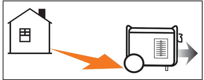
If misused and operated in an unapproved and unsafe location that results in the accumulation of poisonous CO gas inside an enclosed or partially enclosed space, for example a house, garage or a garage with the door partially open, CO Shield® will automatically shut off the generator and then will illuminate a blinking red LED light. **Read the action label for next steps.**
